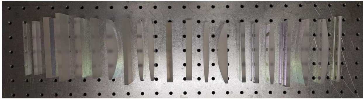
Figure 20. Lenses that are used for the pumping scheme
