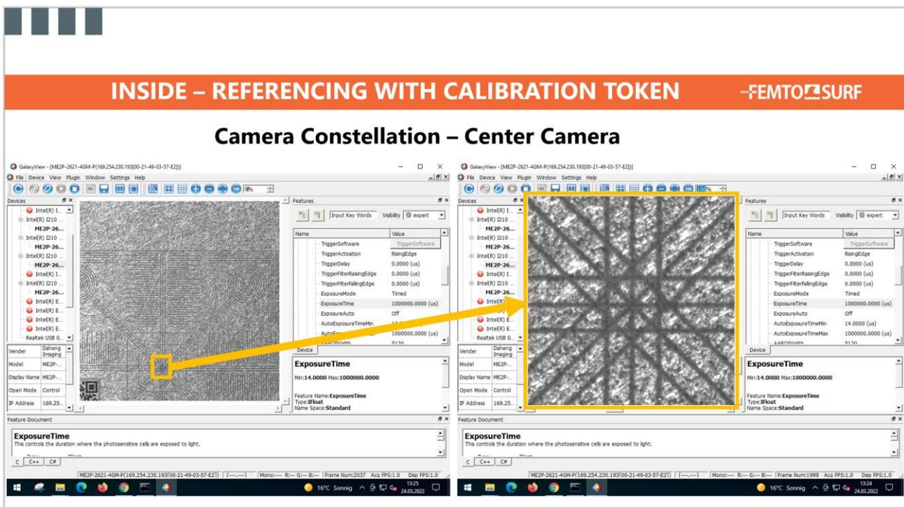
Figure VII: Calibration token scan on FemtoSurf machine with center camera of camera constellation.
