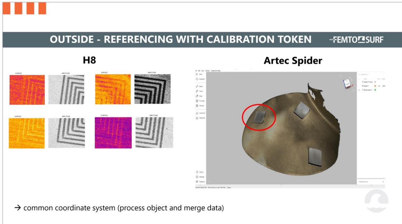
Figure VI: Calibration token scans with H8 (left) and Artec 3D Space Spider (right), ROLLA propeller with calibration tokens attached.
