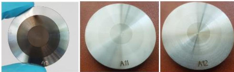
Figure 10. Fabricated 17-4 PH H1025 steel samples for the ball on disk test.
